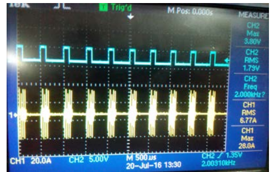
Fig.14. Control pulse of 25% duty ratio and the corresponding tank circuit current
